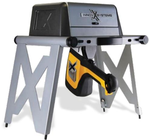
The DELTA workstation with integrated safety-lock shielding can be controlled with a PC.
