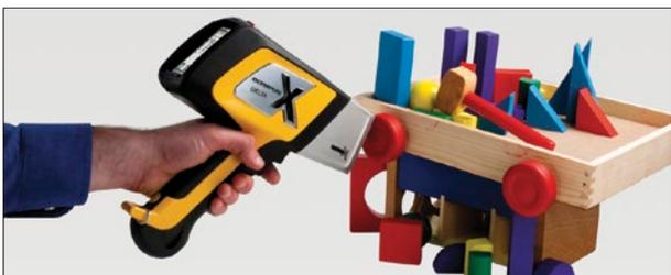
The DELTA can provide positive/negative or pass/fail results for rapid regulatory and safety screening of Pb, Cd, As, Hg, Cr, and other toxic metals in consumer products. Archived DELTA images and results make it the ideal tool for a Reasonable Testing Program.
