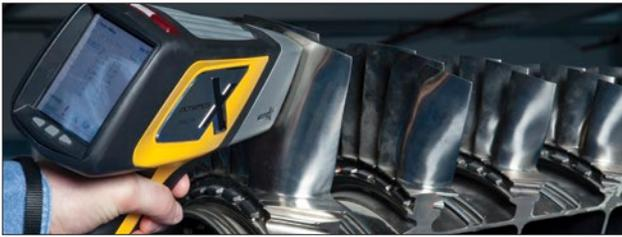
The DELTA can take results and compare them to a library of alloy compositions to “match” an unknown material to known alloys. Pop up messages can be preprogrammed for immediate sorting or coding instructions to increase efficiency and throughput.
